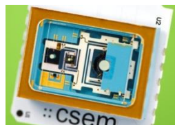
Miniature atomic clock, CSEM, Neuchâtel, 2017 Miniature atomic clock prototype less than 5 mm thick developed by the Centre Suisse d'Electronique et de Microtechnique for the European Space Agency
