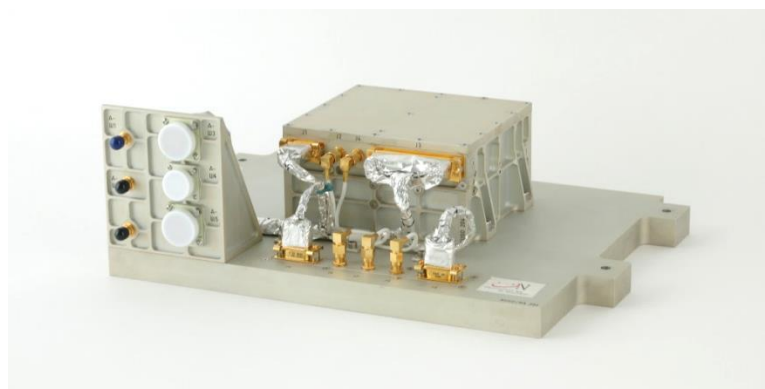
Rubidium atomic clock developed at the Neuchâtel Observatory for the European Space Agency between 1989 and 1994. The clock has been flying since 2011 on the Russian space mission RadioAstron. CSEM, Neuchâtel
